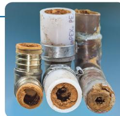
Hard water can clog pipes of any age or type. Here, we can see the dramatic impact calcium and magnesium deposits have in impeding water flow.
